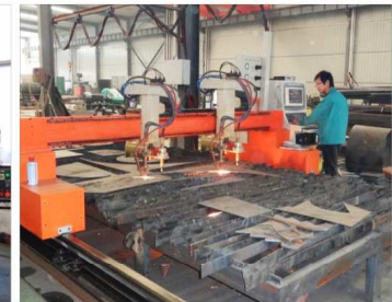
YH-300DHD 数控等离子/火焰两用切割机 CNC plasma/flame and cutting machine
